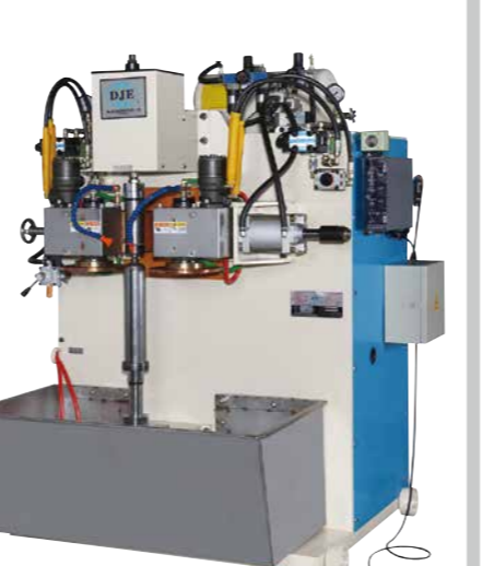
Shock Absorber Seam Welding Machine for Automobile & Motorcycle 汽機車避震器專用輪焊機
