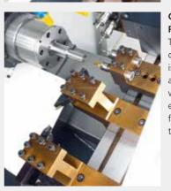
GANG TYPE WITH 2 POSITION POWER TOOLS The gang type tooling system consists of 6 tools. Tool change is fast and conveniently accomplished. This combined with 2-position powered tools enables the machine to perform face milling, drilling and tapping operations.
