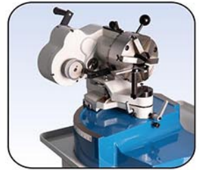
Patent No. 135236 Double cams. It can grind tool of 1/2/3/4/6 Flutes.
